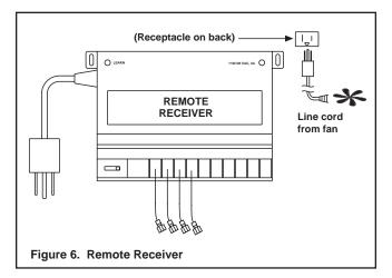
NOTE: The remote receiver will only respond to the transmitter when the 3-position slide button on the remote receiver is in the Remote position. If the system does not respond to the transmitter on initial use, see section Matching Security Codes.
